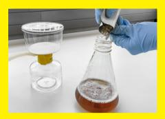
2. Mix to homogenize. Pour the cell culture and filter aid mixture into the Sartolab® RF first, ...
