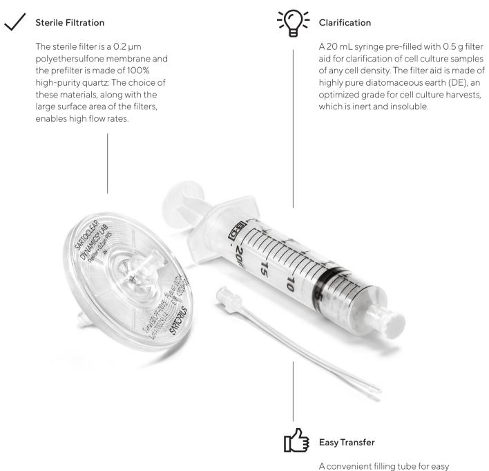
recovery of samples from 50 mL Falcon tubes or Ambr® 15 bioreactors.
