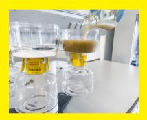
3. Push the Sartolab® filtration unit to apply vacuum to the unit and to start the filtration (second click).
