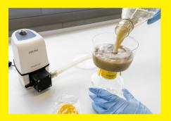
3. ... then filter by simply using the pump.
