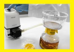
4. After 5 – 15 min., the sample will be available for subsequent downstream processing steps, such as protein purification and concentration.
