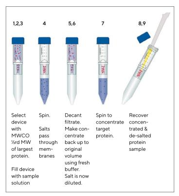
Figure 1: Step-by-step method for desalting and concentration
