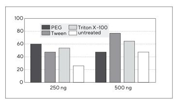
Figure 3: Protein recovery (250 and 500 ng BSA) with Vivaspin $^{\odot}$  2 PES 10 kDa after passivation
