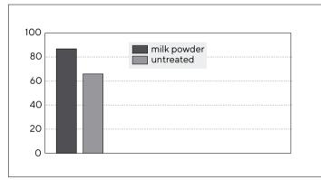
Figure 2: Protein recovery (10  $\mu\text{g}/\text{ml}$  BSA) with Vivaspin® PES 10 kDa after passivation
