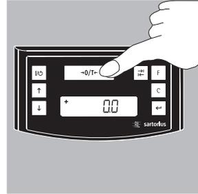
If a different value is displayed: Tare the scale using the
