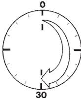
Always allow approximately 30 minutes for the scale to warm up after connecting it to AC power and before performing calibration/adjustment.
