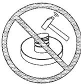
Never use a hammer to close a paint can while it is still on the load plate, as this will damage the weighing system.
