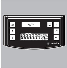
Once the scale has been turned on, it will run an automatic self-test. This is concluded with the readout **0.0** g.
