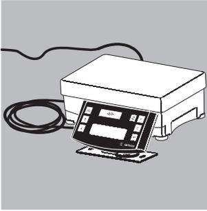
You can calibrate/adjust the scale by pressing the  $\boxed{\rightarrow 0/T \leftarrow}$  key (Zero/tare) (3).
