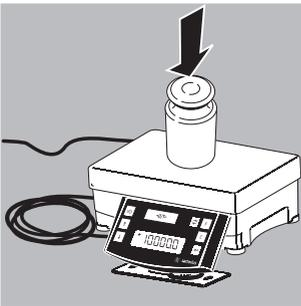
Center the calibration weight on the load plate (15). Adjustment is performed automatically. Remove the calibration weight.
