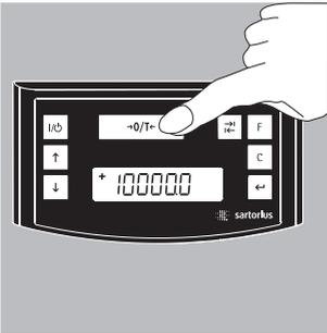
Press the  $\boxed{\rightarrow 0/T \leftarrow}$  key (Zero/tare) (3) for 2 seconds; "10000" is displayed. Release the key.
