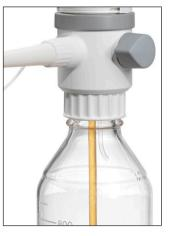
Media Recirculation System Biotrate is equipped with a media recirculation system that allows unused media to be recovered from the device and returned to the bottle. This ensures easy priming and minimizes the media loss.
