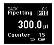
M10 indicates that the pipetting program shown has been saved in memory place 10.
