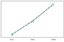
In 3-point adjustment, 10%, 50% and 100% of maximum volume are used to match actual and target results
