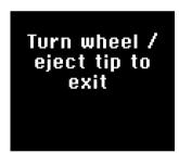
To exit Blow-out, turn the adjustment wheel or eject the tip by pressing the tip ejector button.
