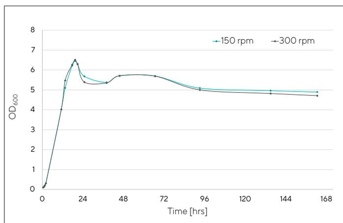
**Figure 6.** Growth curve of *C. sporogenes* cultured at pH 7.0 with continuous feeding and a stir speed of 150 rpm or 300 rpm.
