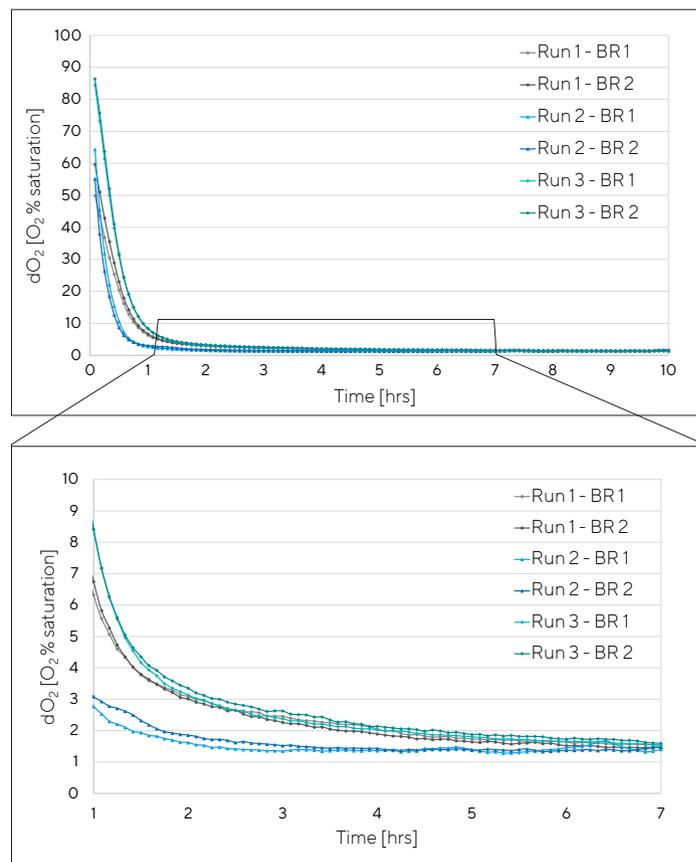
**Figure 3.** Monitoring of  $dO_2$  values under Ambr® 250 self-regulation using two bioreactors (BR) simultaneously during three consecutive runs.
