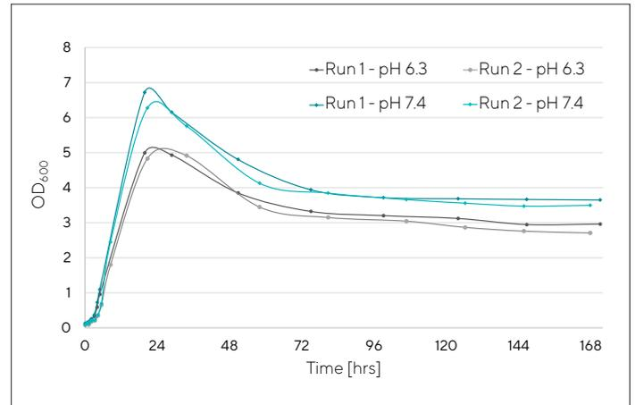
**Figure 4.** Growth curve of *C. sporogenes* simultaneously cultured at pH 6.3 and at pH 7.4 in two Ambr® 250 bioreactor vessel. The experiment was run in duplicate.
