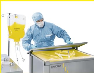
Pre-designed Solutions for storage and shipping of buffers used for purification or final formulation
