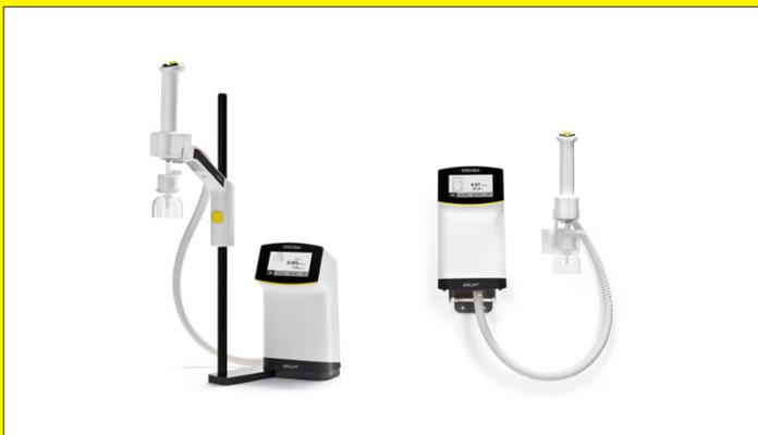
Adapted to your needs, the Smart Station has two installation options: wall-mounted or bench top.
