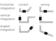
→ Direction of flow Flow Sensor
