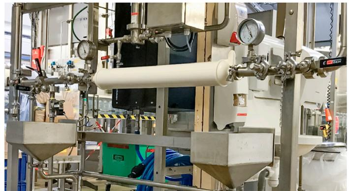
Figure 5B: Process Flow With Sterilizing-Grade Maxicaps Installed
