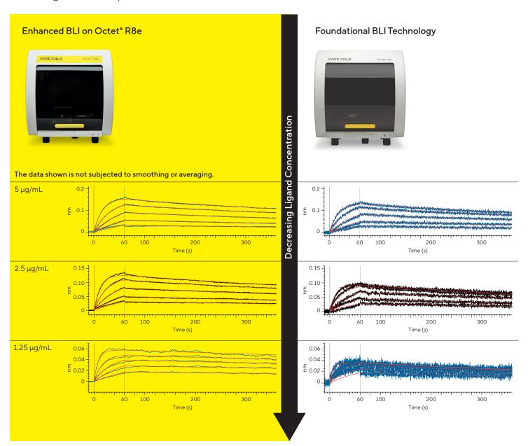
The Octet® R8e BLI System delivers cleaner data with significantly lower-noise levels.
