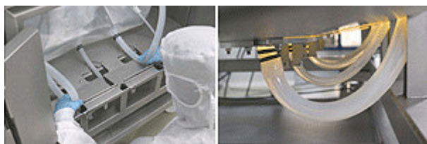
Pre-connected mixing loops
