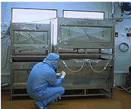
Buffer solution storage and distribution for chromatography in 200L and 500L customised Palletanks®. Connections made using portable LAF cabinet.
