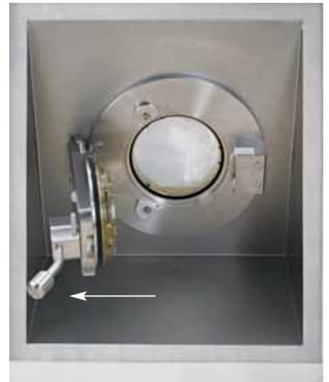
Inside Opening: Handle to allow the Biosafe Port opening from inside.
